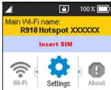
1) LCD Screen: indicates signal strength, WiFi Name, Wi-Fi Password, number of devices connected, and data usage.
