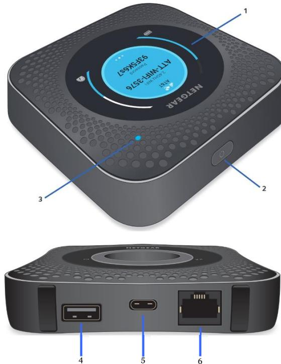
1) LCD Screen: indicates signal strength, WiFi Name, Wi-Fi Password, number of devices connected, and data usage.
